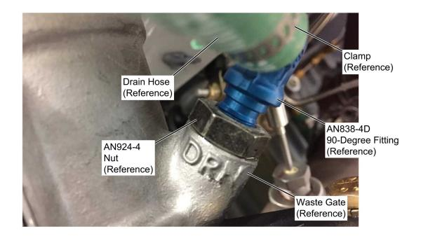
Figure 1. O-RING INSTALLATION FOR TURBOCHARGER WASTE GATE OIL DRAIN LINE (Sheet 1)
